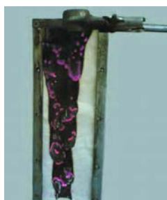
Fig. 1 Mostashari's Flammability Tester with a low addition of sodium borate deca-hydrate applied onto a cotton fabric just before the end of the experiment. Uneven burned and carbonaceous areas in the fabric are shown in the figure
